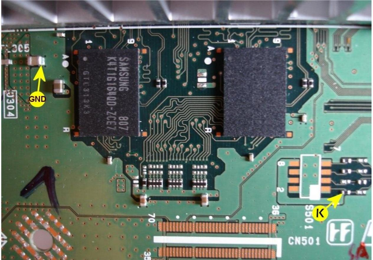
Stick the logic board on top of the two RAM chips with some double sided tape.
